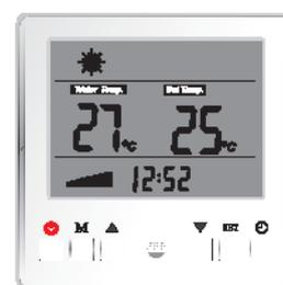
Picture shows that heating and hot water mode is selected
